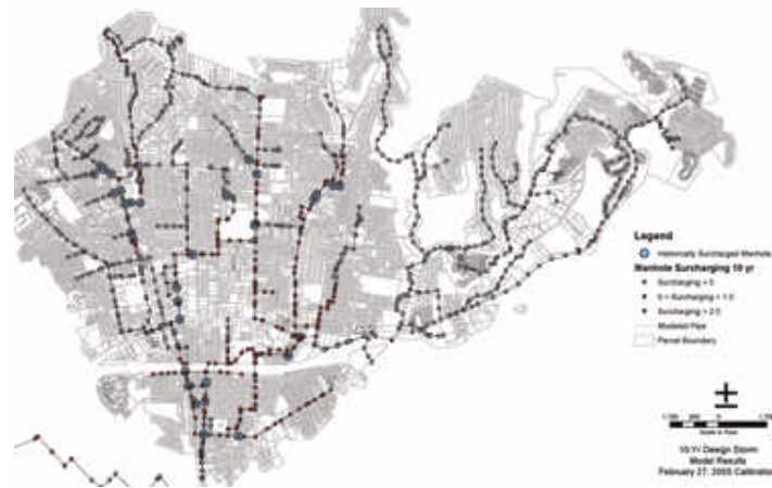
10-year storm model with historically surcharged manholes.
